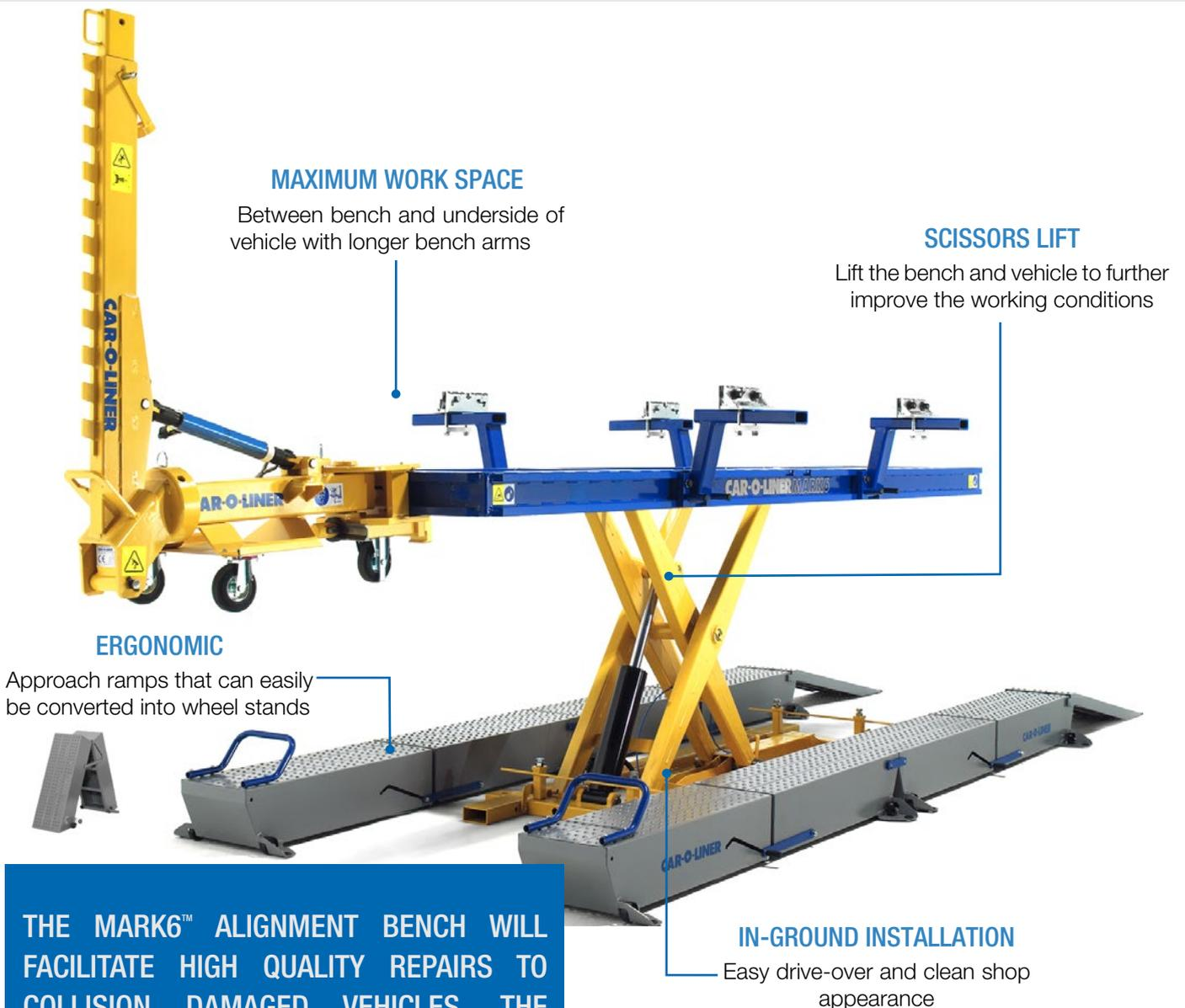
THE MARK6™ ALIGNMENT BENCH WILL FACILITATE HIGH QUALITY REPAIRS TO COLLISION DAMAGED VEHICLES. THE BENCH IS SUITED FOR MOST PASSENGER CARS AND LIGHT TRANSPORT VEHICLES.
